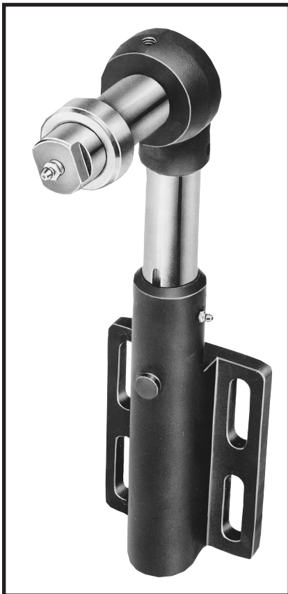
A spring loaded tensioner; this one is in a piston arrangement, similar to a pneumatic tensioner. The idler head rotates completely, and slots in the cast base allow linear adjustment.
